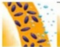
In a vacuum the rice loses all the air contained in it. In the following warm water bath the nutrients start to become soluble and move out of the husk.
