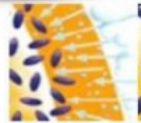
To move the nutrients out of the husk, but inside of the rice, the hot steam and air pressure is used (otherwise the nutrients would just get washed out into the water).
