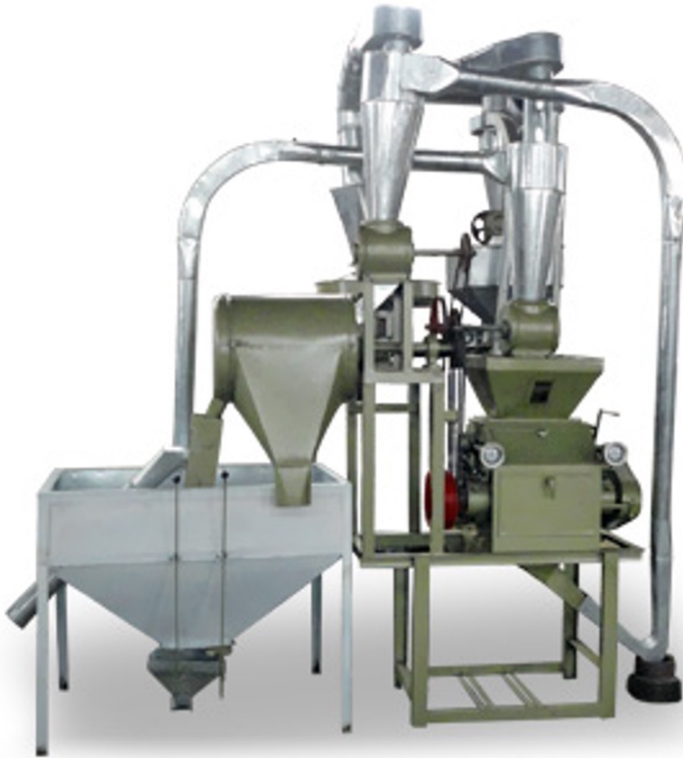
A small-sized mill for wheat flour production
