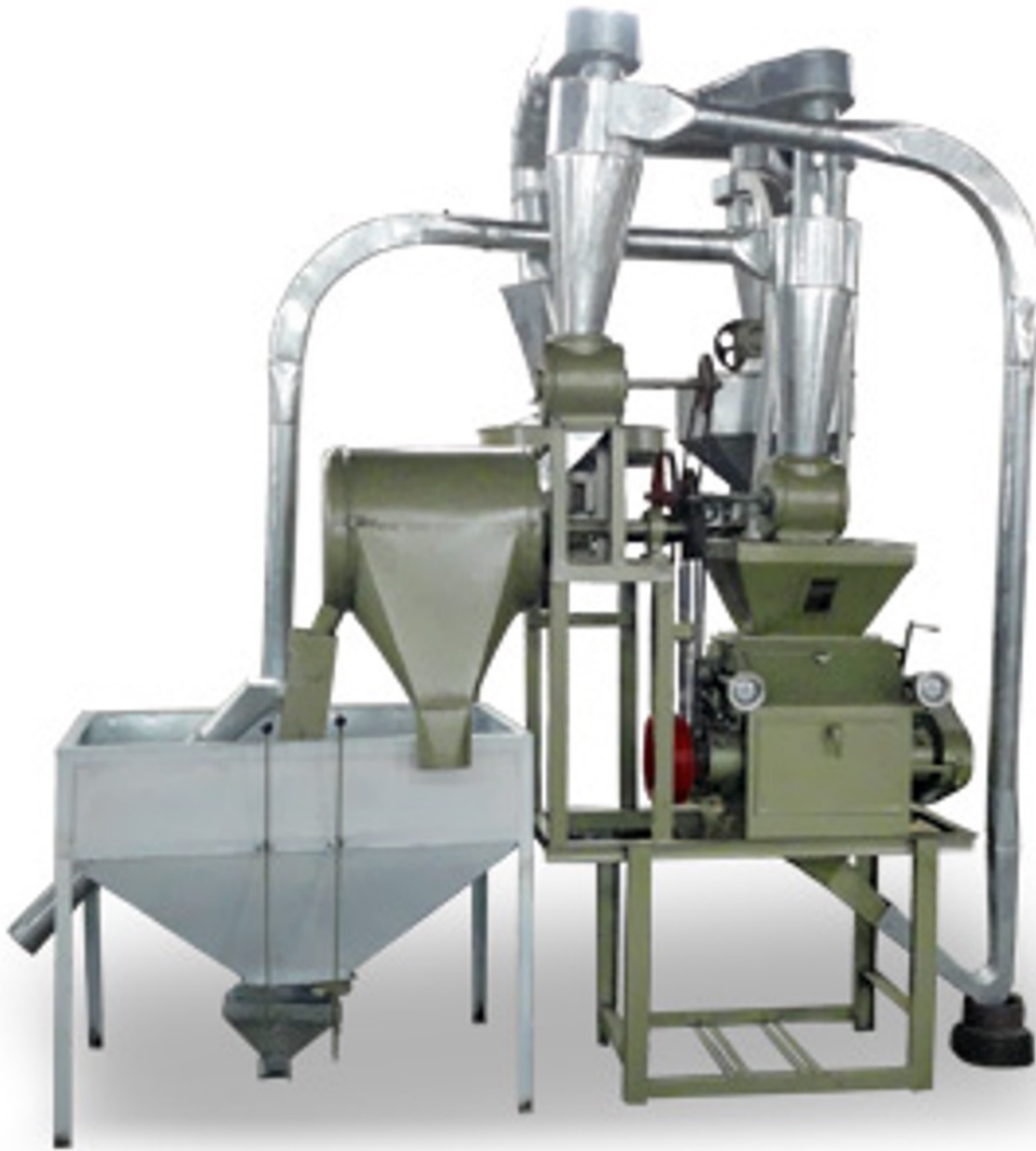
A small-sized mill for wheat flour production
