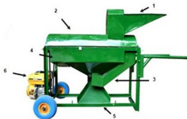
The thresher consists of a 1) feed chute, 2) threshing chamber, 3) exit chute, 4) blower, 5) seed collection chute, and 6) petrol engine
