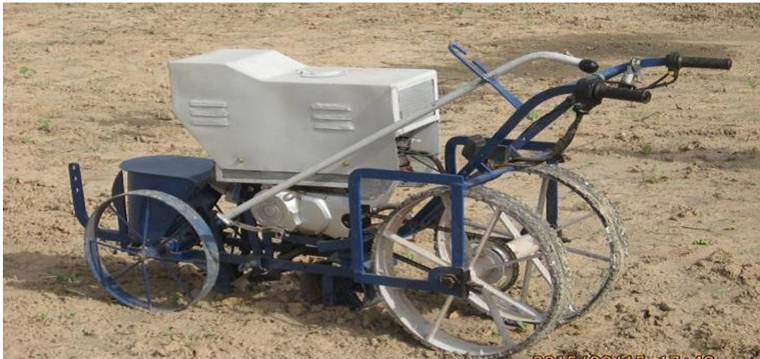
Sénékéla planter and micro-dose fertilizer applicator
