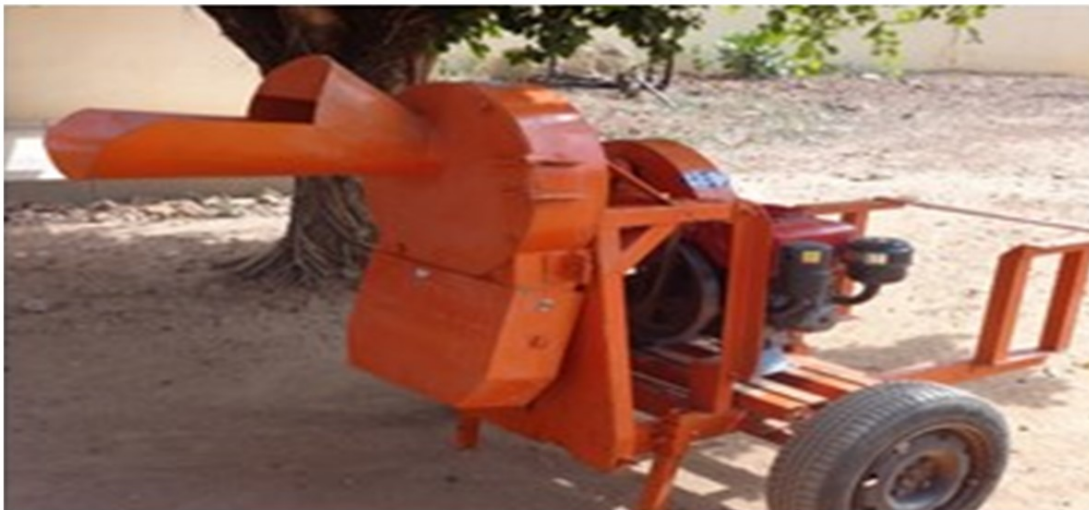
Forage chopper with in-built engine
