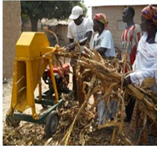
Use of motorized stover cutter (left) and mobile chopper (right)
