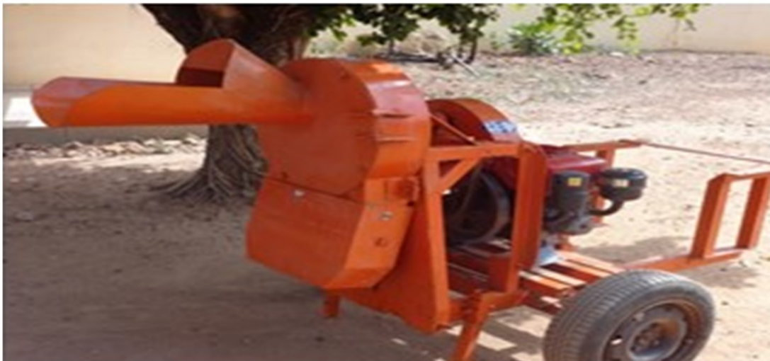
Forage chopper with in-built engine
