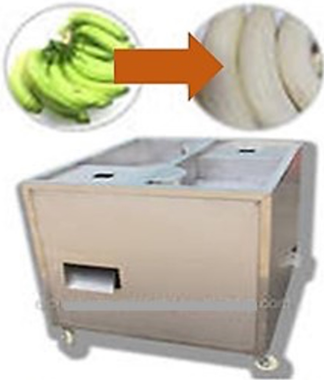
An industrial green banana peeler able to processes 600 units per hour
