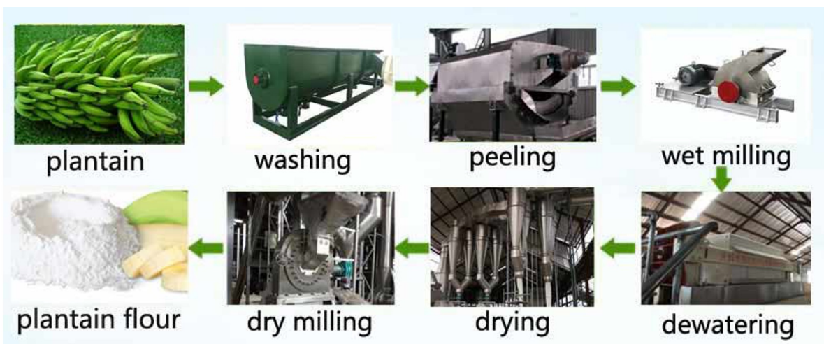
Steps of industrial flour production from plantain (Credit: Kaifeng Sida)
