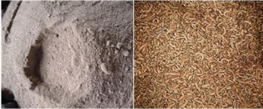
*Feed formulation before (left) and after dry extrusion (right)*
