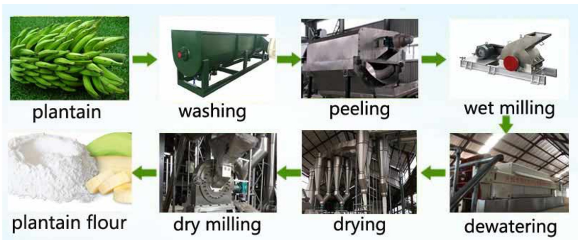
Steps of industrial flour production from plantain (Credit: Kaifeng Sida)
