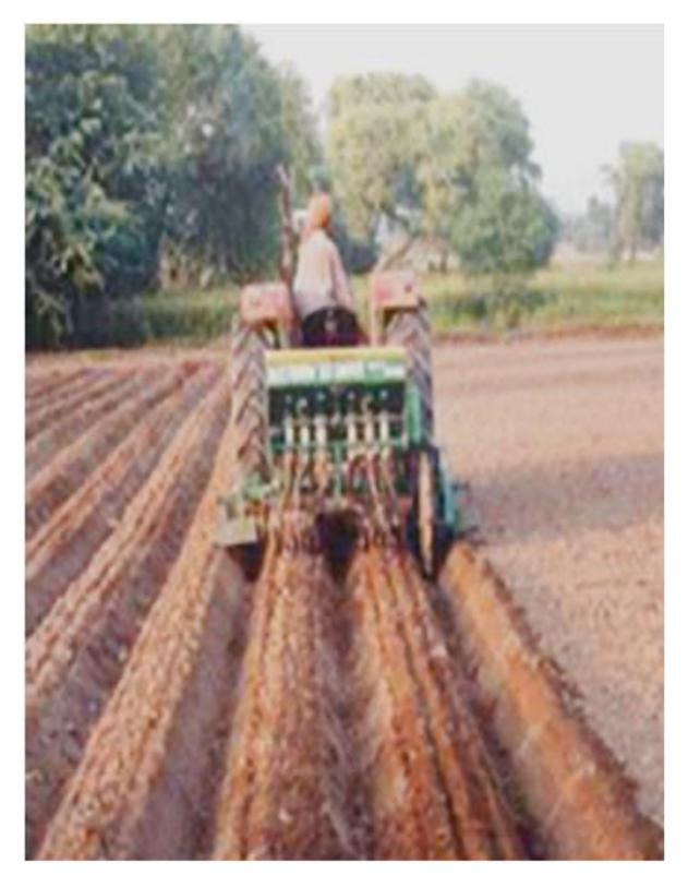
Establishing raised beds, furrows and planting rows in a single pass over a tilled and level field
